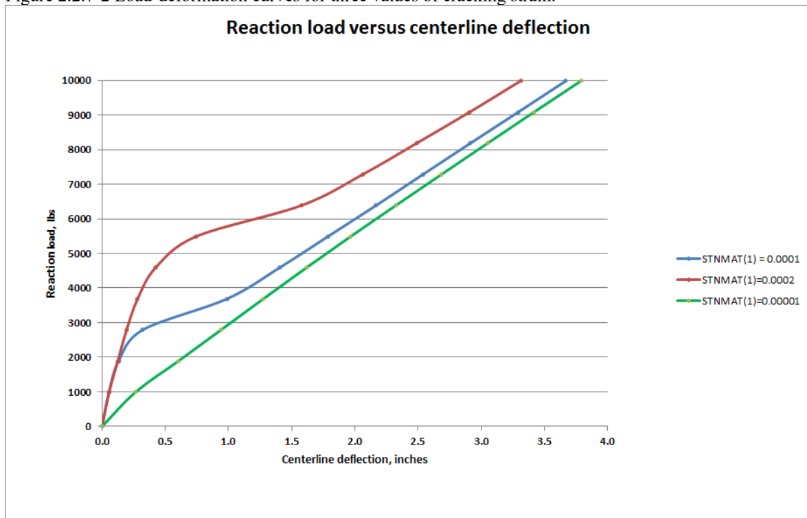
Figure 2.2.7-2 Load-deformation curves for three values of cracking strain.
